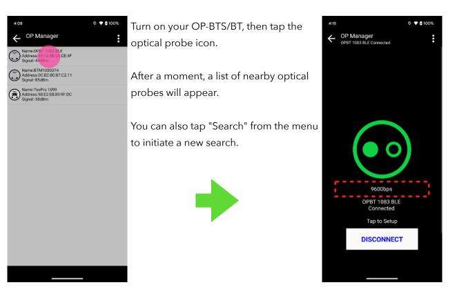
Select the device you want to connect to. The optical probe icon will turn green, displaying the device name and baud rate below it.
